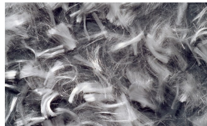
Fibrin XT BS EN 14889 Class 1a Micro Monofilament Fibre at 0.910 Kg per Cubic metre of concrete
