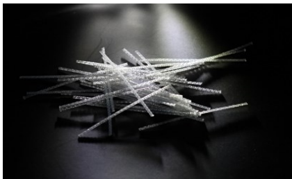
Durus Macro fibre BS EN 14889 Class 2 Embossed at 5Kg per Cubic metre of concrete
