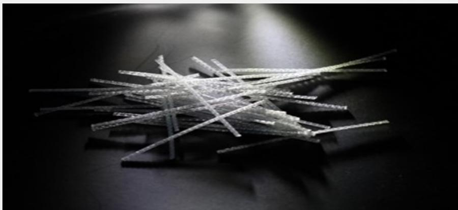
Effective replacement of conventional steel mesh reinforcement in marine concrete applications.
