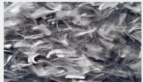
Fibrin XT BS EN 14889 Class 1a Micro Monofilament Fibre at 0.910 Kg per Cubic meter of concrete
