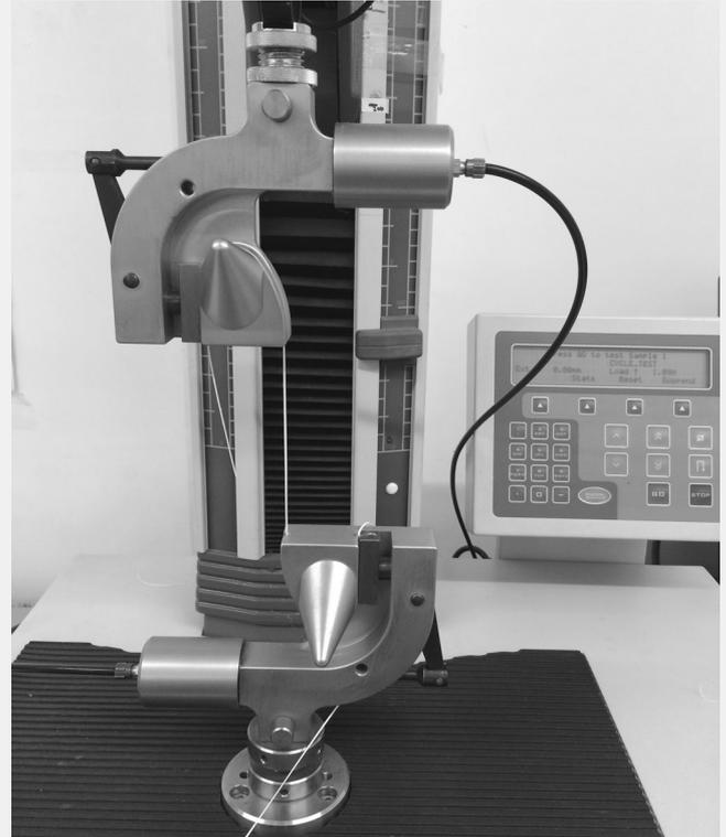
Tensile test of Durus® S500 filament according to EN
