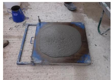
**Concrete Flow test to ensure workability**
