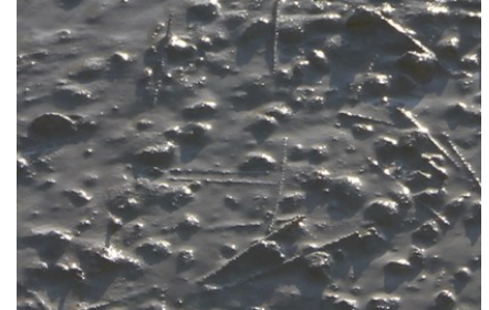
Durus S400 macro fibre concrete mix
