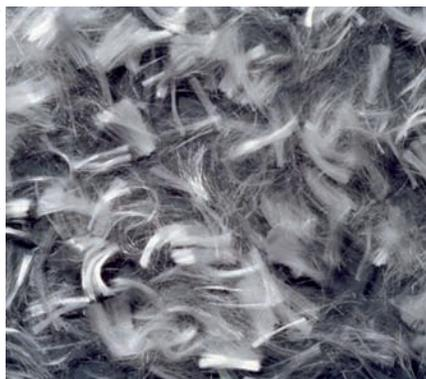
Figure 1: ADFIL polypropylene fibres.
