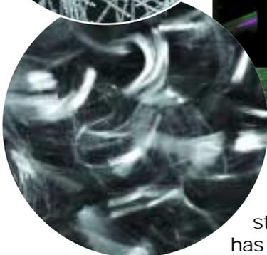
Figure 2 above: Close-ups of polypropylene fibres.
