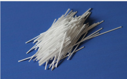
Durus S300 BS EN 14889 Class 2 Embossed Macro Fibre at a 4 kg per cubic meter of concrete.
